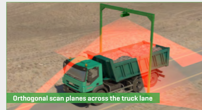
Hardware with two 2D laser scanners, RFID and HD camera
